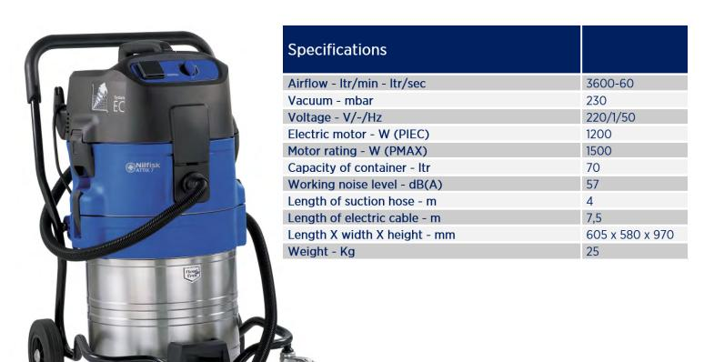
This container type model provides a highly effective means of dealing with a multitude of vacuuming applications involving fine to coarse particle substances such as dust, gravel, wood and metal shavings, etc. as well as non-flammable liquids.
