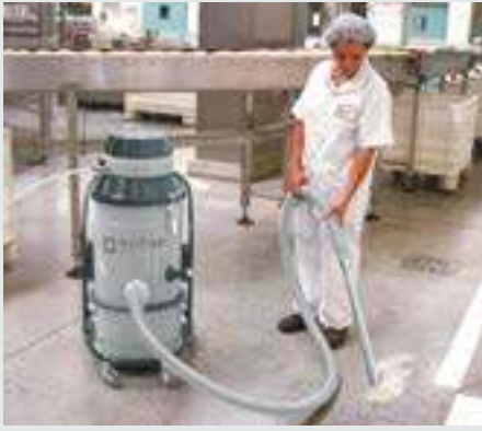
Recovery of flour in ATEX environment.
