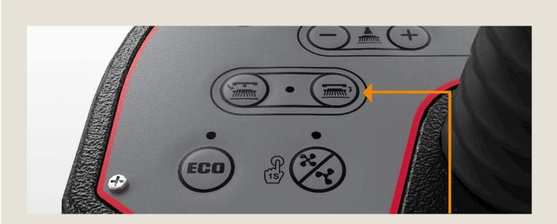
Turn the main key to on and press the click on button to install the brush automatically. Deck will lower and brushes turn slowly to attach.
