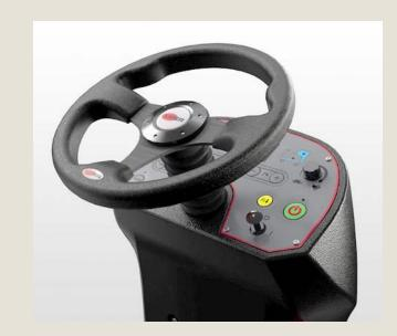
During the cleaning job it's possible to adjust the solution flow, the brush pressure, activiting Eco Mode or Silent Mode from the dashboard.
