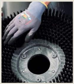
With the key turned on press the brush click off button to remove the brushes/pad holders for inspection and cleaning.
