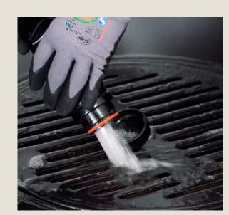
Empty the tank with the hose in the back. Empty and clean the debris tray in the tank, flush&clean out the recovery tank.
