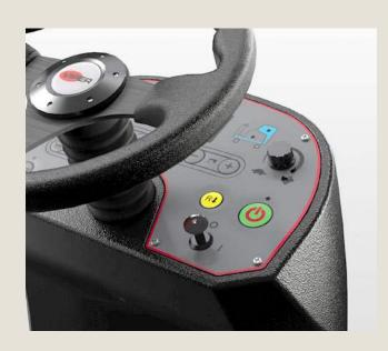
Turn OFF the machine using the key.
