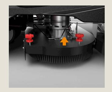
To install the brush/pad holder, pull up the metal handle and slide in the brush/pad holder until it stops against the pins in the proper position and release the handle. Put back the side skirt
